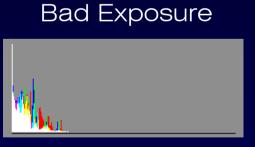
"Thin", under-exposed digital negative. You will need to"push" in post (gain) which will be noisy
