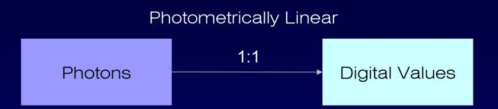
Doubling of light means doubling of digitally encoded value
