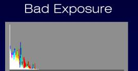
"Thin", under-exposed digital negative. You will need to"push" in post (gain) which will be noisy
